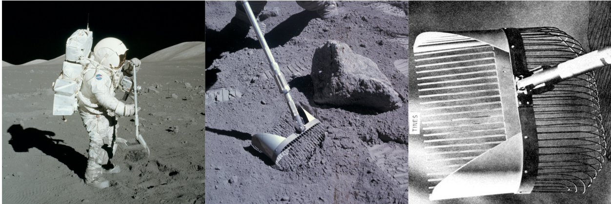
Figure 8.7: The rake used to collect an unbiased sample of small rocks in the lunar regolith. (Left) Jack Schmitt with the rake on Apollo 17 [NASA AS17-134-20425]. (Center) The rake in the lunar regolith from Apollo 16 [NASA AS16-116-18690]. (Right) Close-up image of the rake from [4].
